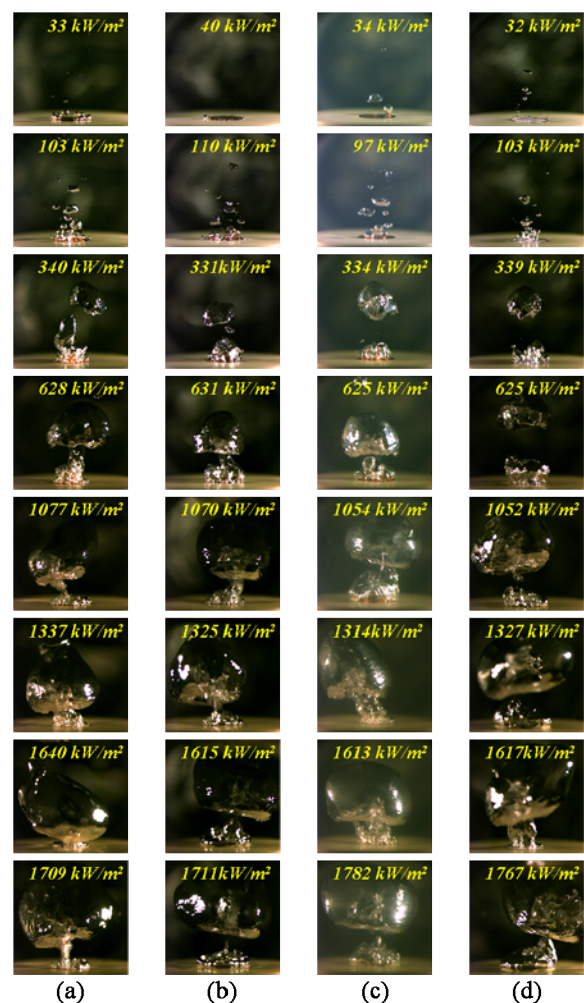
Fig. 11. Visualizations of \text{Al}_2\text{O}_3 nano-fluids with smooth heaters and pure water with coated heaters : (a) Nano-fluids of 10^{-3} g/liter with a smooth heater, (b) pure water with a coated heater of 10^{-3} g/liter, (c) Nano-fluids of 10^{-2} g/liter with a smooth heater, (d) pure water with a coated heater of 10^{-2} g/liter.
